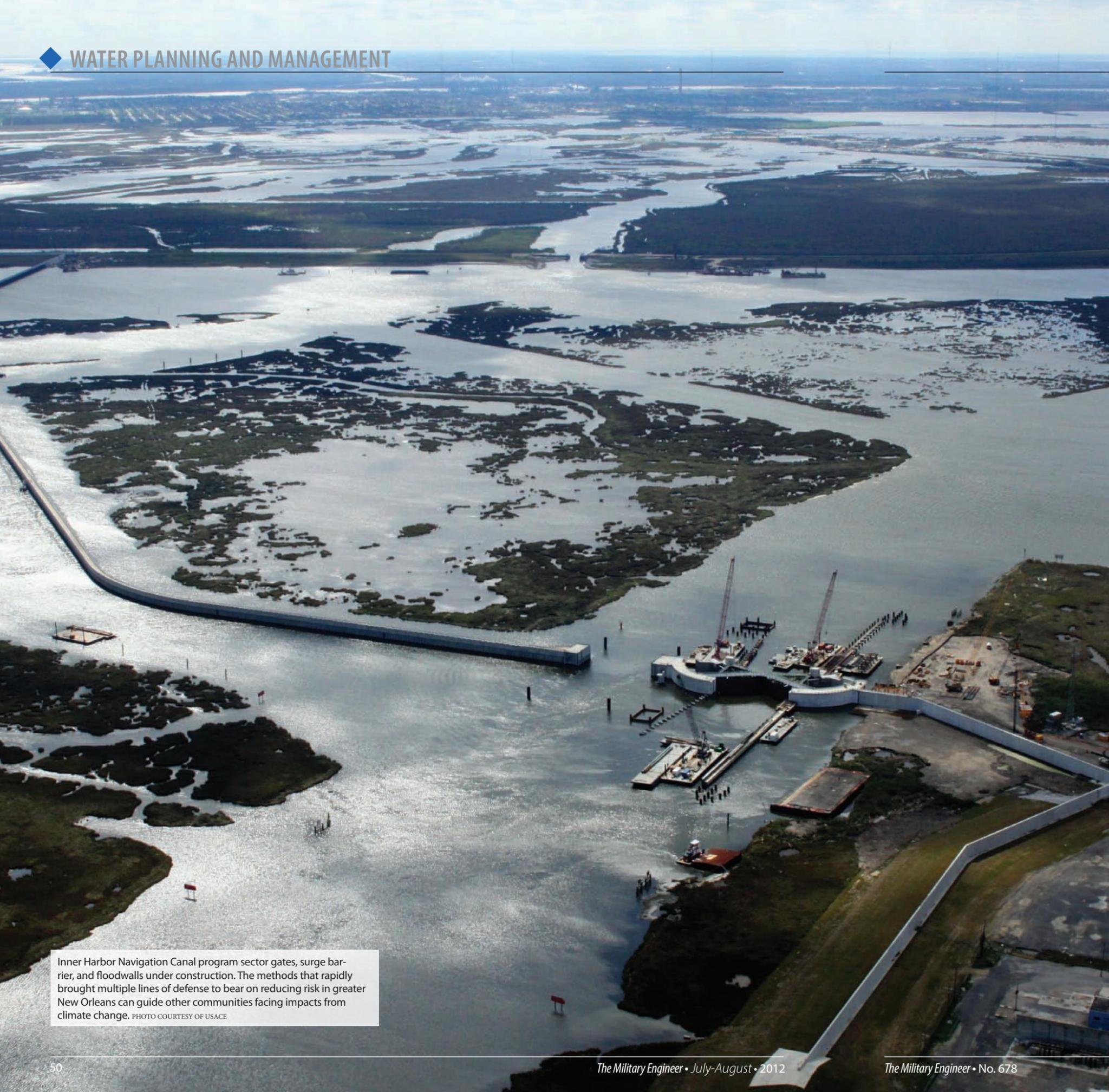
Inner Harbor Navigation Canal program sector gates, surge barrier, and floodwalls under construction. The methods that rapidly brought multiple lines of defense to bear on reducing risk in greater New Orleans can guide other communities facing impacts from climate change. PHOTO COURTESY OF USACE
